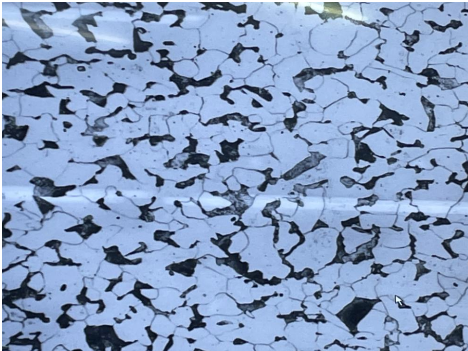
Figure 2: Micrograph of the work hardened EN3 (1015) specimen
